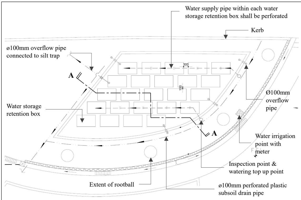
Diagram 3 – Sample of zero irrigation system
