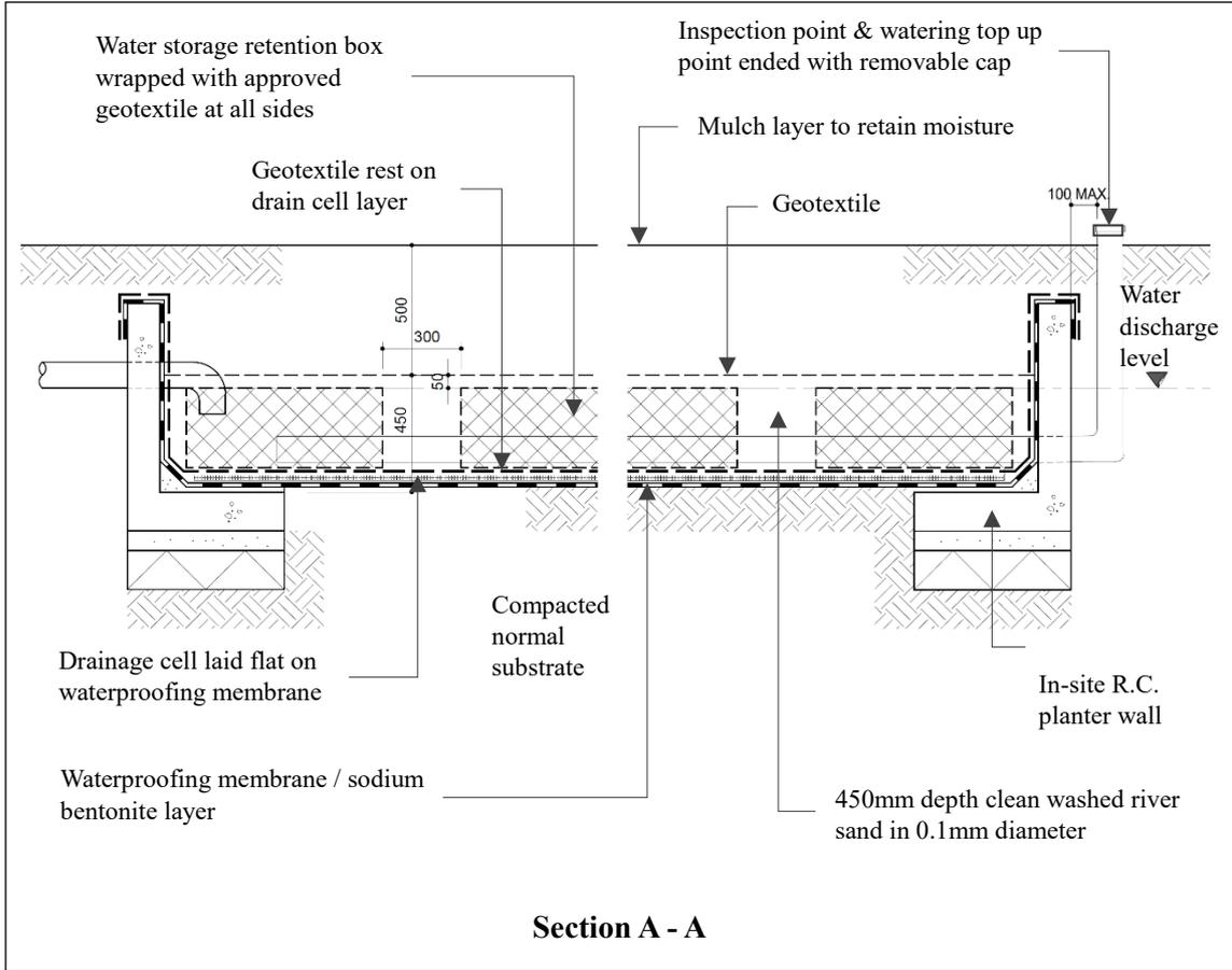
Diagram 4 – Sample of zero irrigation system
